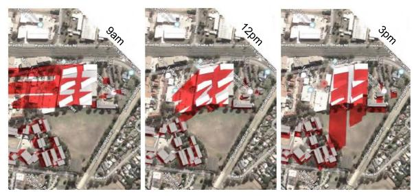
Figure 12: Shadow diagram during winter solstice.
